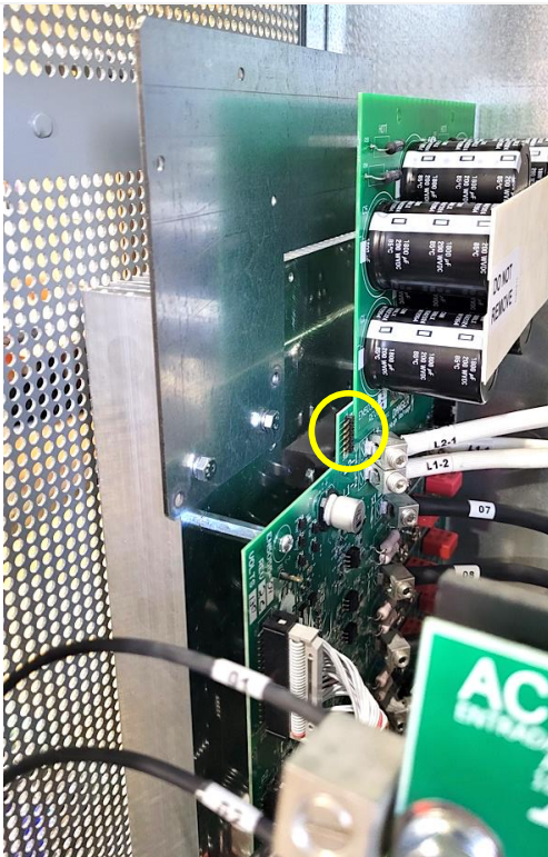
Figure 1A – Location to Connect Auxiliary I/O Board with Power Board
