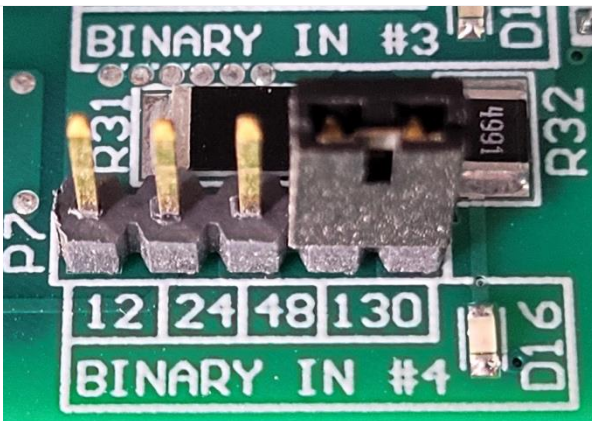
Figure 11A – Binary Input Jumper #4 with Factory-Default of 130 V
