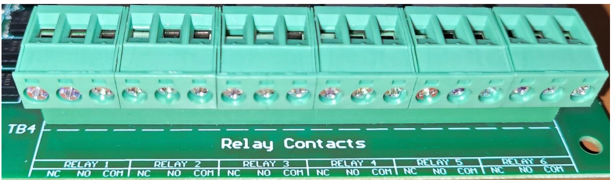
Figure 4 – Terminal Block for Relay Connections
