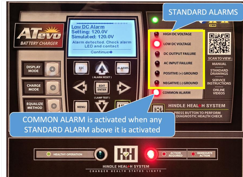
Figure 3 – Standard (Legacy) Alarms & Common Alarm
