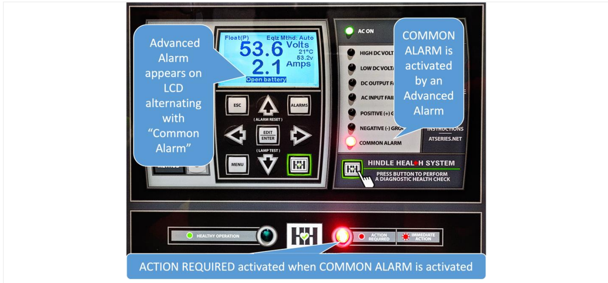
Figure 5 – Advanced Alarm That Triggers the Common Alarm
