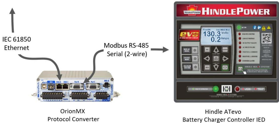
Figure 3 - Connections between Orion Protocol Converter the ATevo charger
