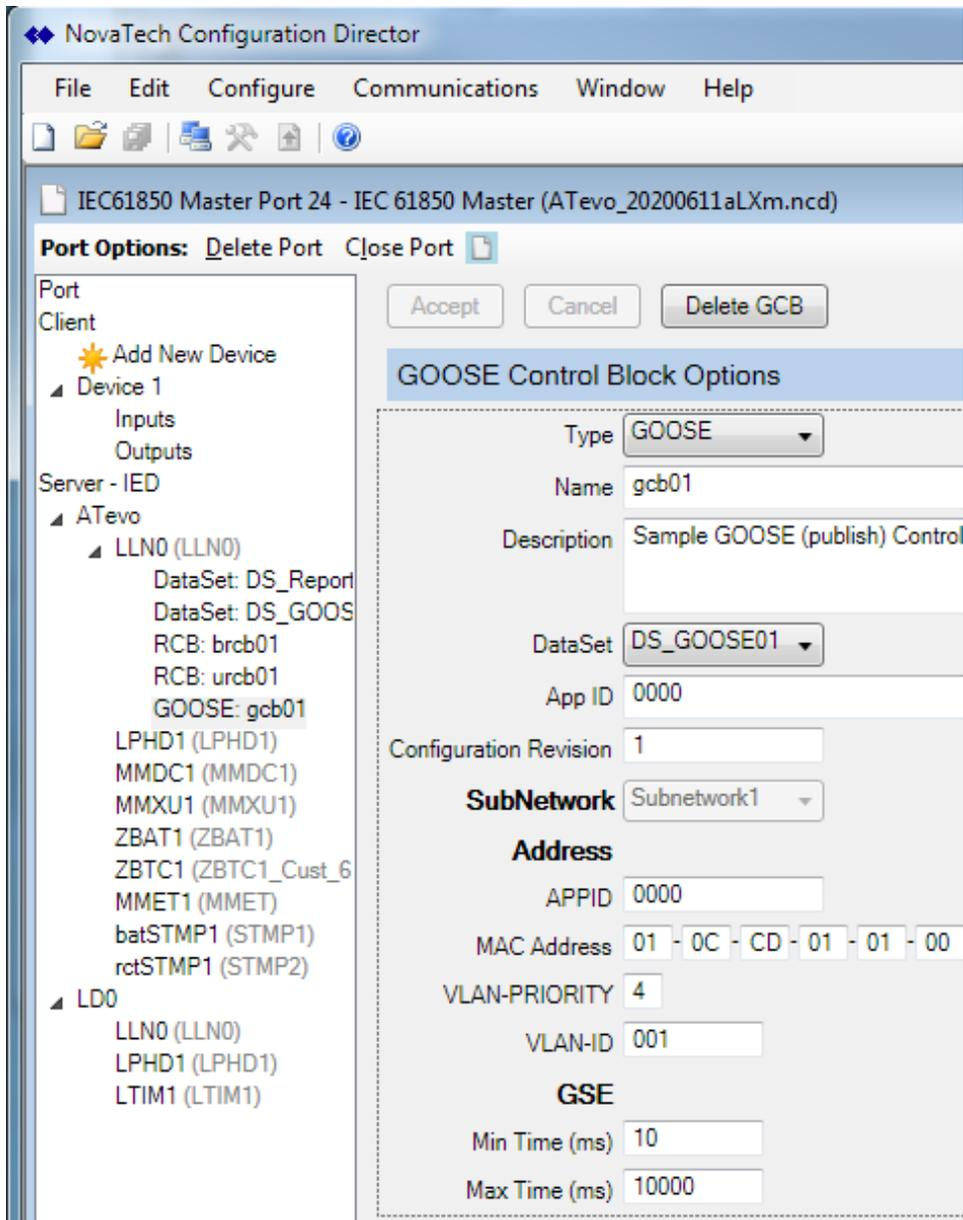
6. Configure IP address if needed (for top-down, IP address was already imported)
