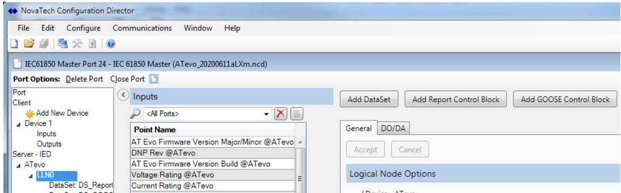
Note that GOOSE “addressing” is configured when ATEVO/LLN0/“GOOSE:” is selected. The Destination (GOOSE multicast) address is indicated by “MAC Address”. The APPID is the value 2-byte value inside GOOSE Ethertype header. The “App ID” is the name of the GOOSE (also known as GOOSE ID or GoID). VLAN-ID also needs to be configured to match the subscriber expectation.
