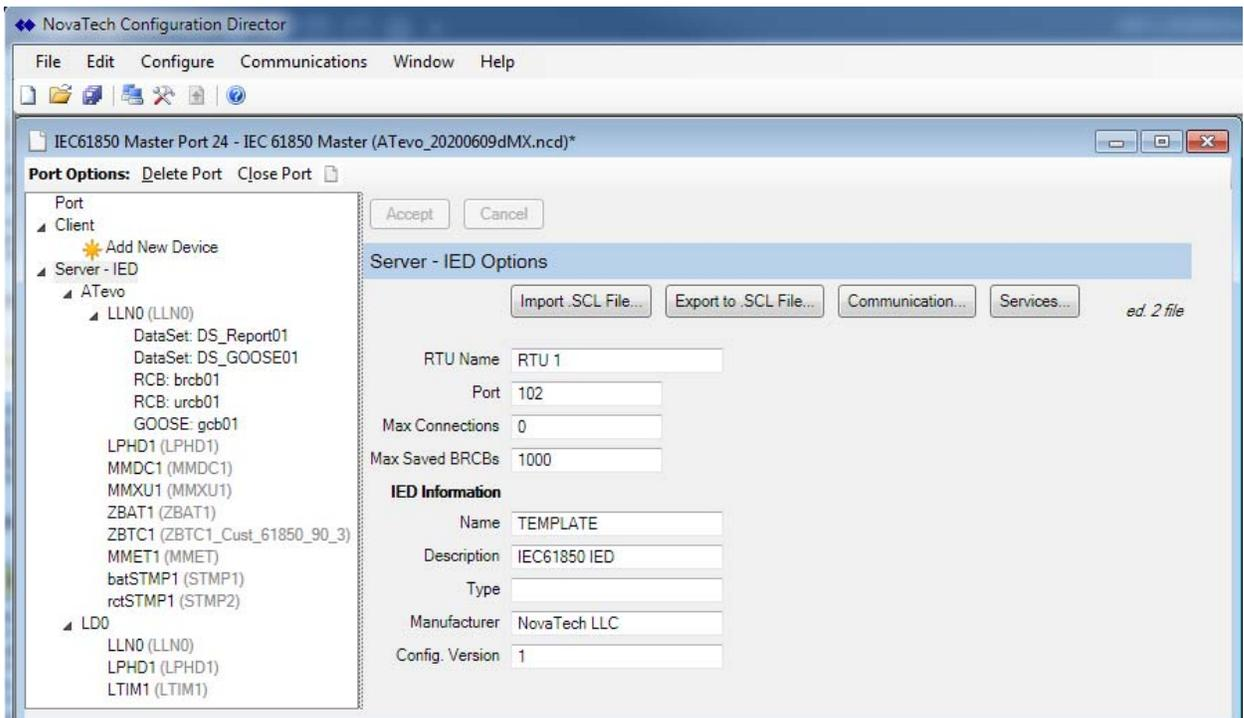
The default file has 2 datasets, a buffered RCB, an unbuffered RCB, and a GOOSE.
