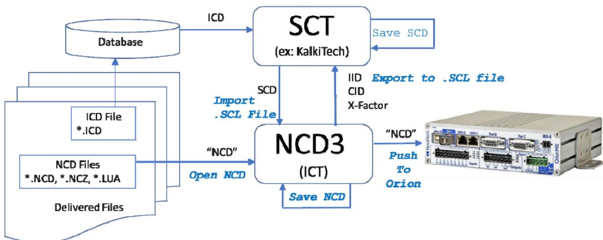
Figure 5 – IEC 61850 Configuration Workflow
