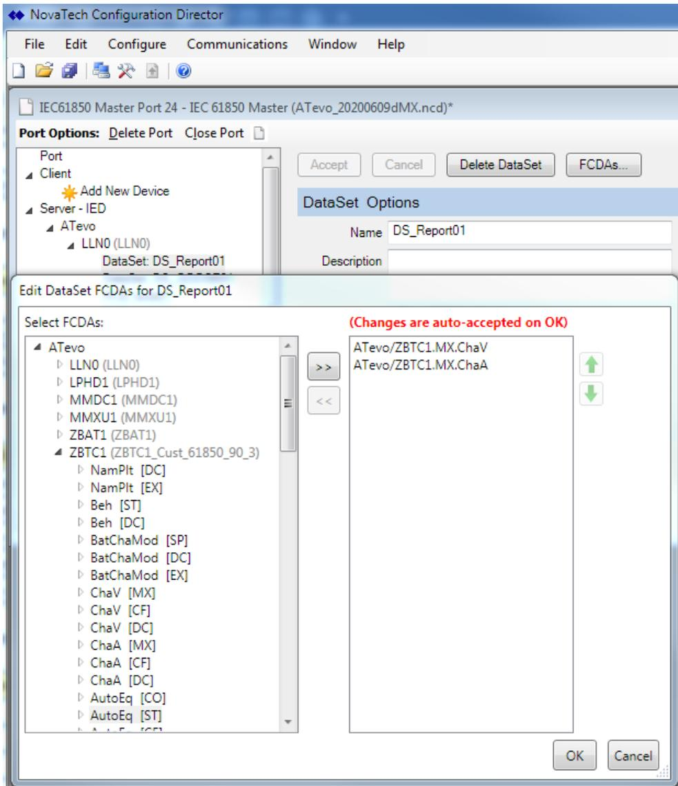
This shows that “AutoEq (ST)” has been selected and pressing the “>>” key would add it to the DataSet. Similarly, an object on the right pane could be selected then “<<” to remove it from the dataset. The number of elements in a DataSet is limited to 250 elements for a Report and possibly fewer for GOOSE (limited by the maximum Ethernet packet size).
