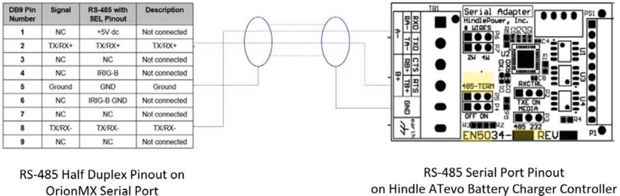
Figure 4 – RS-485 2-wire Connections between Orion Protocol Converter and ATevo charger
