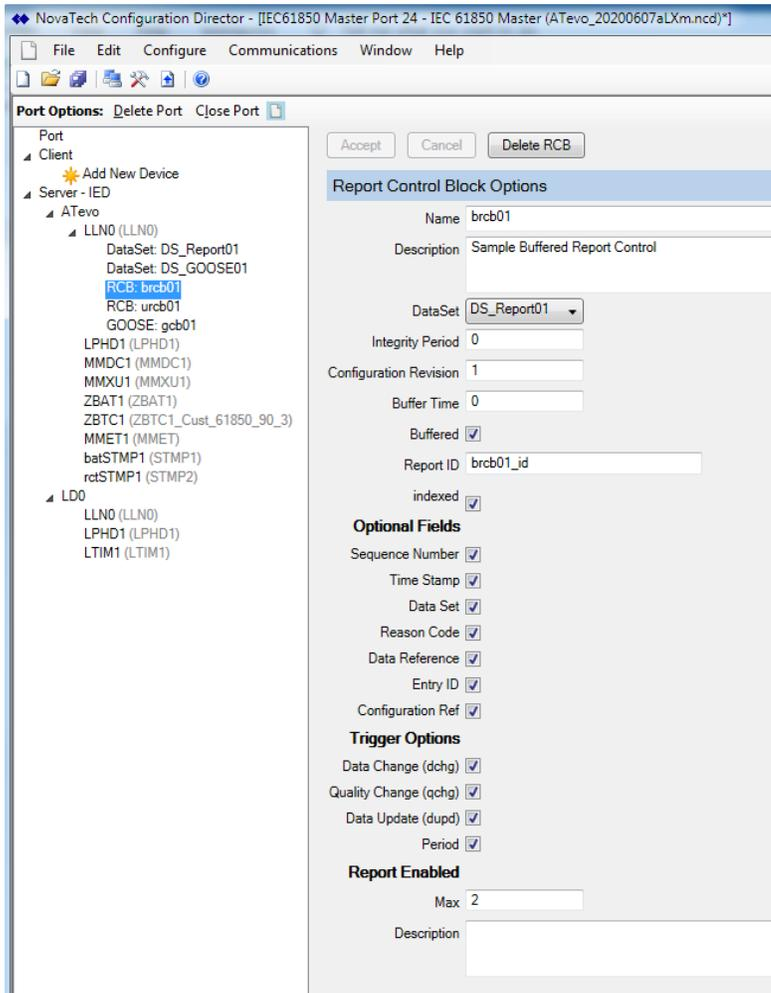
Figure 1 – Initially configured Functional Constraints, DataSets, Report Control Blocks and GOOSE
