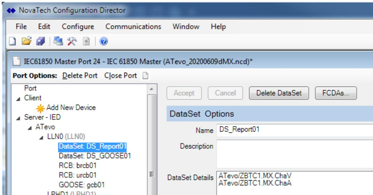
Here we see 2 elements in the dataset, the battery charger output voltage and current.
